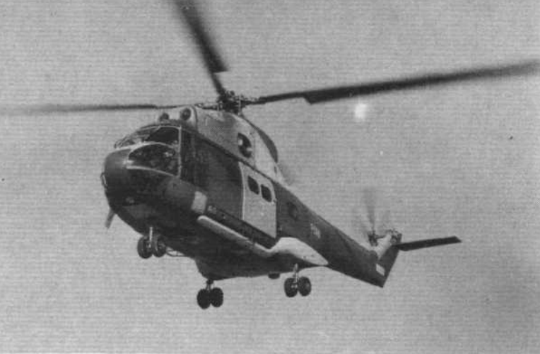
First of the Package Deal The first production Sud-Aviation SA.330 flew recently for the first time at Marignane. It shows a number of changes from the pre-production aircraft, which have been flying for some time; notably, the addition of a stabiliser on the tail-rotor boom. Westland contributes much of the structure for the SA.330, which is the first of the three helicopters in the Anglo-French package deal
