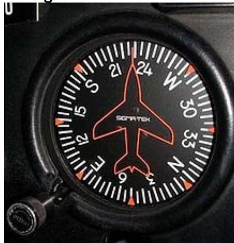
This Gyrosopic Compass can be set manually before flight and then monitored for compass alignment during flight, it can of
