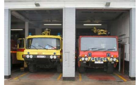
Two of the Fire and Rescue vehicles stand ready for immediate call out. The Yellow vehicle is a light foam/rapid intervention tender, Carmichael Jet Ranger, Scammell propelled by a Cummins VTA 903 V8 Turbo Charged Intercooled Diesel Developing 500BHP with an Allison Automatic Four Wheel Driven with Super Low Gear and diff lock.
