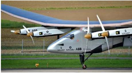
This Solar powered aircraft is currently making some extensive flights. It is able to charge its batteries during the day from the 17,000 solar panels on its upper wing surfaces driving the electric engines.
