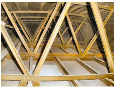
The construction of the centre section ribbing continued to the outer section and filled with fuel which gave the 2,500nm range.
