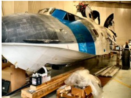
The fuselage is released from its large wing after 70 years and is being prepared for trestling, even so the minimum width of the hull is 10ft 6" when the wheels are retracted. The length remains at 61ft and height at 14ft or a bit less.
