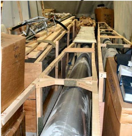
Outer wing section components packed with special heat treated wood for shipment to USA, a customs botanic regulation.
