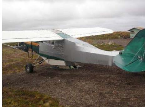
The skills and ingenuity of this bush pilot are to be admired – the advantages of a metal framed aircraft are evident, for this get you home repair with available products such as duct tape. A monocoque wooden constructed aircraft would have been destroyed beyond repair. The Hurricane fighter of WW11 was easily repaired for the same reason because of the metal tubing employed in its construction and covered with fabric. This aircraft was flown safely back to base.
