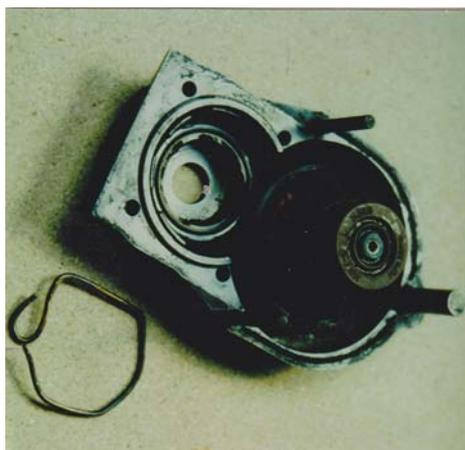
Pictured (*column one*) is a picture of the first magneto in which a cir-clip came loose, when the second magneto shaft sheered, the errant cir-clip managed to get jammed and rejuvenate the first magneto back to life again. A safe landing was made without fuss.
