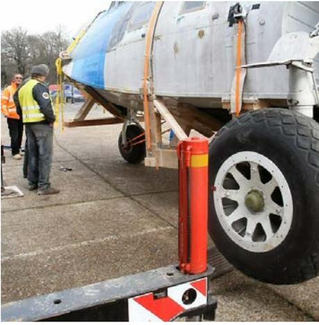
Testing the initial lift for loading from the wing attachment point was a little bit nose heavy. Removing the nose wheel corrected this problem perfectly.
