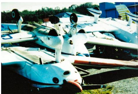
Good formation to the bitter end...! These aircraft were secured to the concrete by their wing points, which were no match for the strength of the hurricane.
