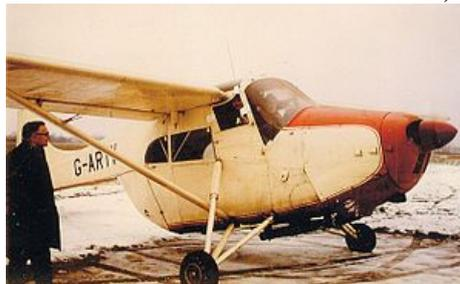
It was fitted with a 6 cylinder 295HP engine whilst some were fitted with 375HP Armstrong Siddley Cheetah engines.
